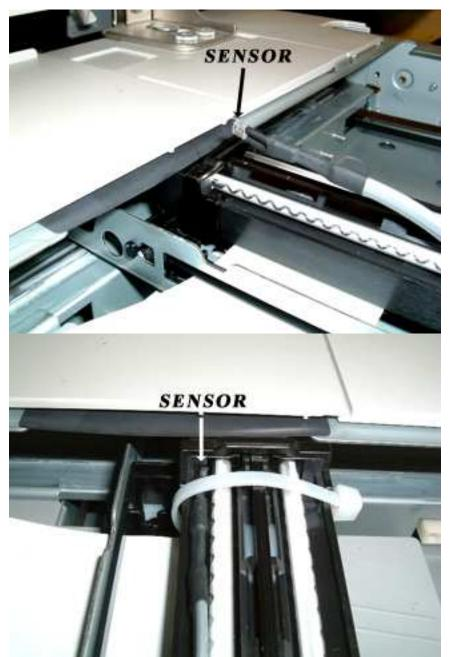
Please note the sensor is held in place with a small ty wrap provided for you in the kit. The ty wrap must be installed in such a way that it does not drag or rub anywhere.
